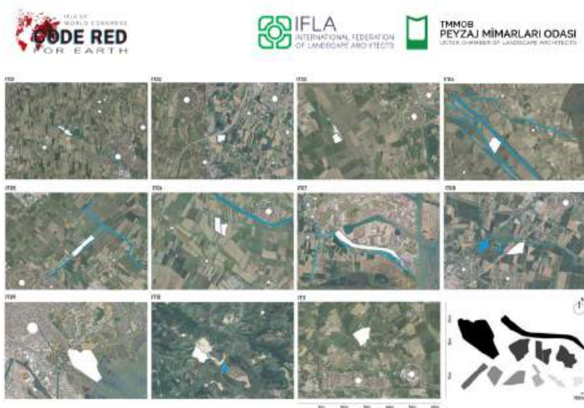
Figure 9. “Thick” mapping analysis of landfills in Italy in relation to water bodies, settlement centers and infrastructure (background-aerial photos: Google Earth Pro)
